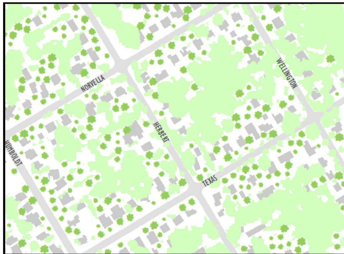
Each tree icon represents a possible tree planting location that avoids buildings, underground utilities, and other infrastructure. Tree spacing is 30 feet.
