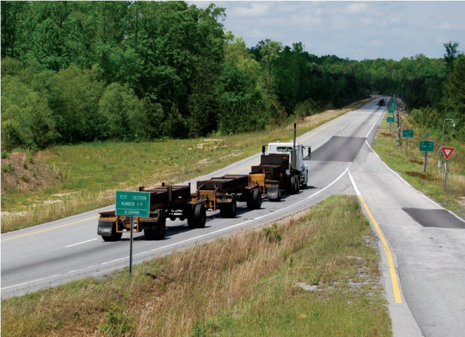
A truck on the warm-mix test track at the National Center for Asphalt Technology.
